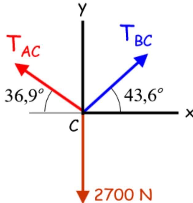
$$R_x = 0 \therefore T_{BC} \cos 43,6^\circ + T_{AC} \cos 143,1^\circ + 2700 \cos 270^\circ = 0$$
