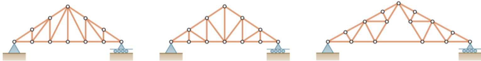
Typical Roof Trusses
